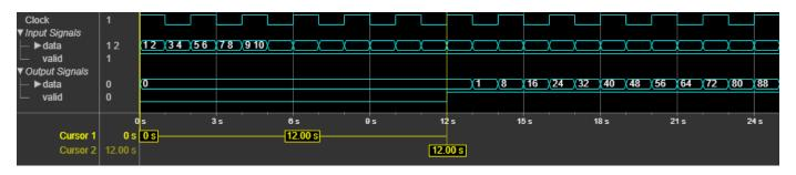
This figure shows the output of the System object for an eight-element column vector input with a fixed decimation rate, R, M, and N values of 8, 1, and 3, respectively, and GainCorrection set to true. The latency of the object is 44 clock cycles.
