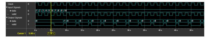
This figure shows the output of the System object with a fixed decimation rate, DecimationFactor, DifferentialDelay, and NumSections values of 8, 1, and 3, respectively, and GainCorrection set to true. The System object returns valid output data at every eighth cycle based on the fixed DecimationFactor value of 8. The latency of the object is 15 clock cycles and is calculated as 3 + N + 9.
