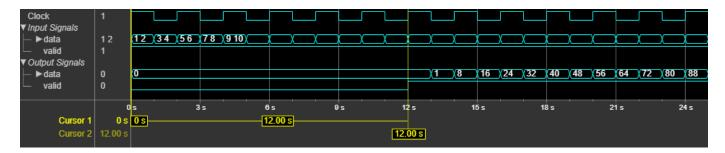
This figure shows the output of the block for an eight-element column vector input with a fixed decimation rate, R, M, and N values of 8, 1, and 3, respectively, and the **Gain correction** parameter selected. The latency of the block is 44 clock cycles.
