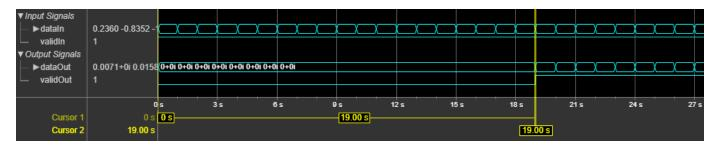
This figure shows the output of the block for a vector input of length 8 when you set the **Filter structure** parameter to **Direct form systolic** and all other parameters to their default values. The latency of the block is 31 clock cycles.
