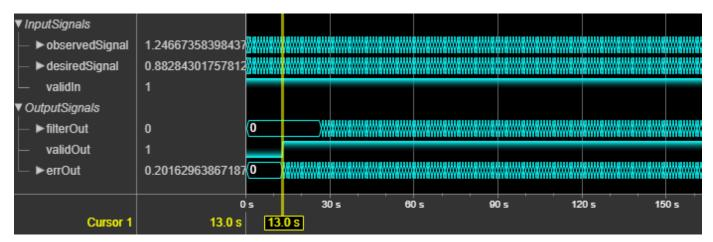
This figure shows the output of the System object for a 4-by-1 real vector input when you set the FilterLength argument to 64 and all other properties to their default values. The latency of the System object is 18 clock cycles.
